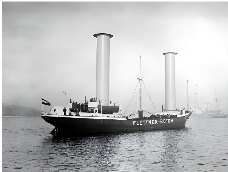
Figure 1. Anton Flettner's first Rotor ship, the Buckau [15].
